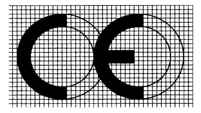
If the "CE" conformity marking is reduced or enlarged the proportions given in the graduated drawing set out in this point must be respected.
